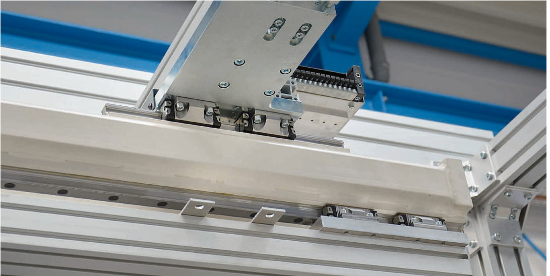
Gantry for handling sleeves. The X axis is moved by a dual linear module with a KU 30.30 recirculating ball bearing guide
