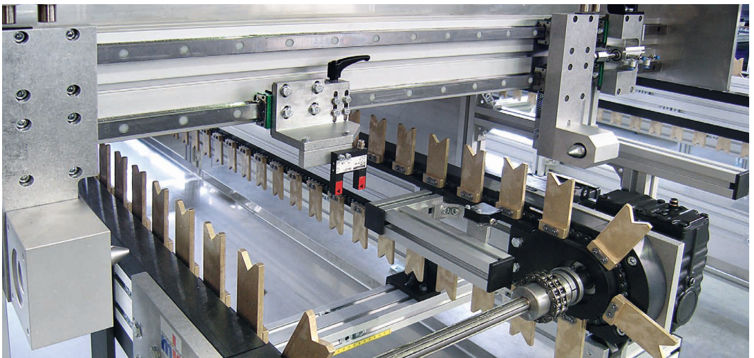
Recirculating ball bearing guide for manual lane width adjustment and for clamping the pneumatic centring device and electromotive rotating unit
