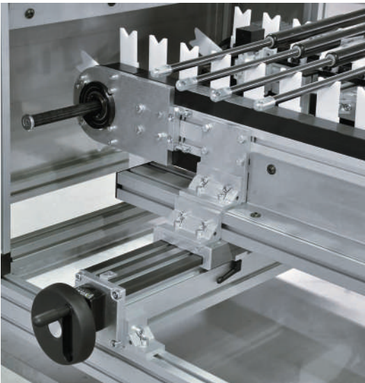
VST 2011 adjusting unit used for semi-automatic conveyor width adjustment in a chain conveyor system
