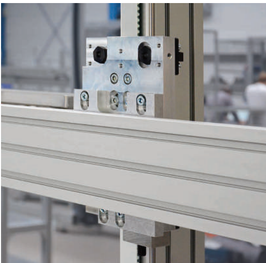
Linear unit LZR 2004-38.41-30 as a height adjustment unit for an assembly and testing workstation
