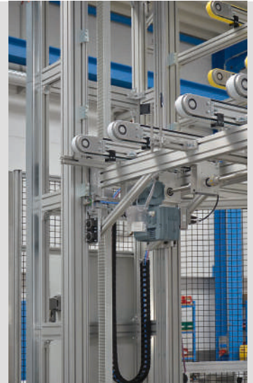
Lift for storage system
