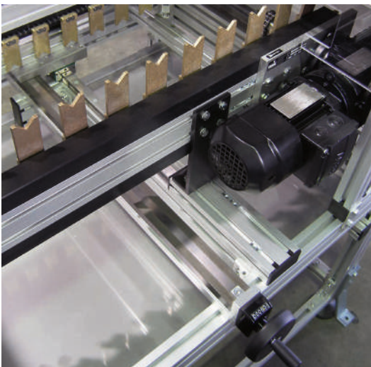
Dual VST 2015 with parallel recirculating ball bearing guide for supporting the load
