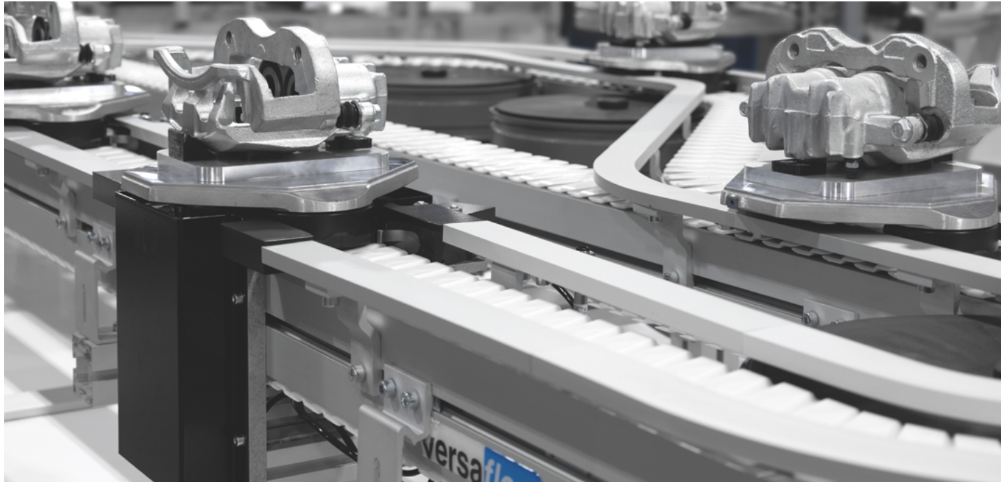
A pallet is entering into the Lift and Locate Module. First the pallet will be stopped using a Pallet Stop positioned within the Lift and Locate Module.
