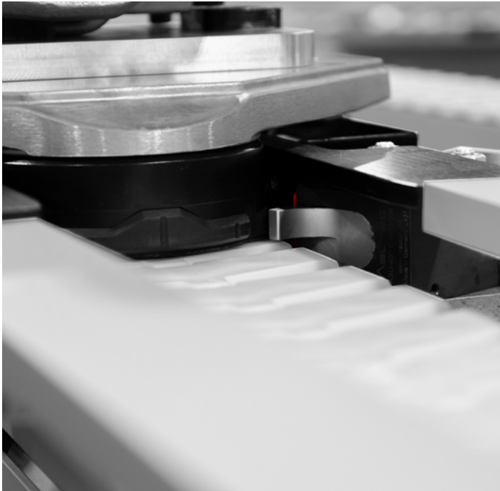
A close up view of a pallet stopped via a Pallet Stop.
