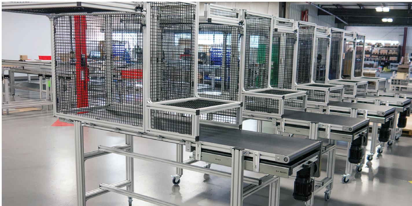
Conveyors from mk North America, like these GUF-P 2000 Belt Conveyors, can easily be modified to include a variety of accessories, such as safety guards.
