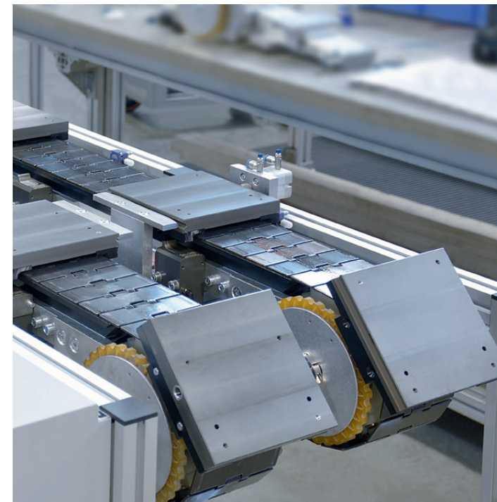
SPU 2040 Recirculating Pallet-Handling Conveyors can be designed to carry one or two rows of pallets.
