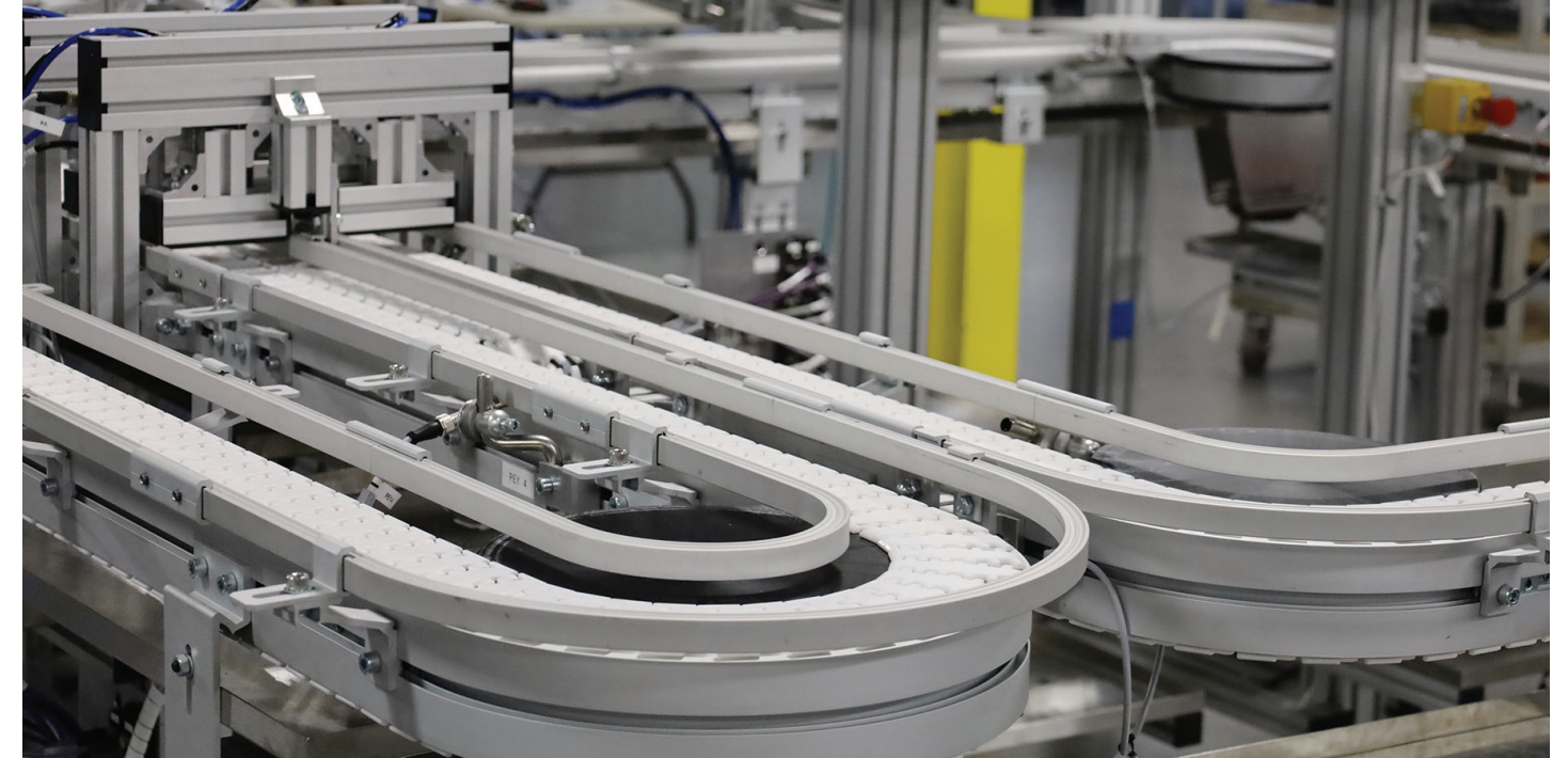
VersaFlex conveyors are ideal for conveying product in multiple directions and to multiple destination locations.
