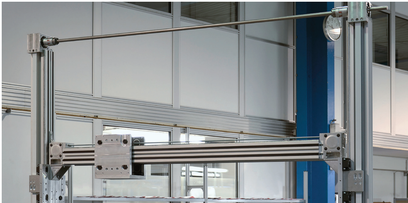
In this example a dual-axis linear module comprised of an LZR 2011 with a side-mounted carriage plate.
