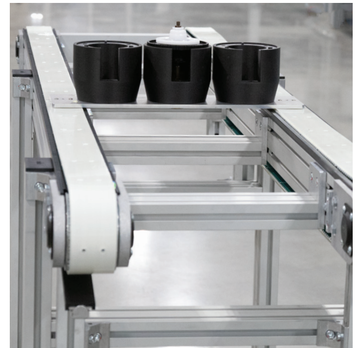
Inserts are placed into Timing Belts, this allows fixtures to be bolted to the belt, as seen in this example.
