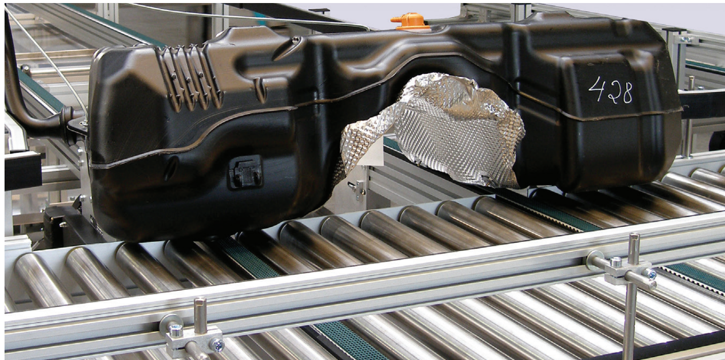
Roller Conveyors are ideal for transporting oversized parts. Timing Belt Conveyors are used to transfer parts between perpendicular Roller Conveyors.
