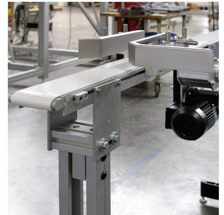
Here a GUF-P MINI Belt Conveyor with a center drive is customized with side rails unique for the application.
