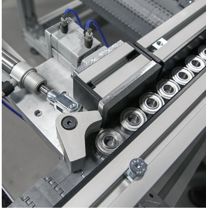
Parts can be metered off of a conveyor line using a pneumatic escapement.
