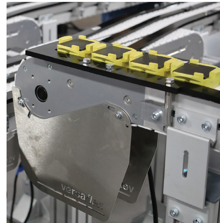
VersaFlex conveyors can be used to convey product, pallets or pucks – depending on the application.
