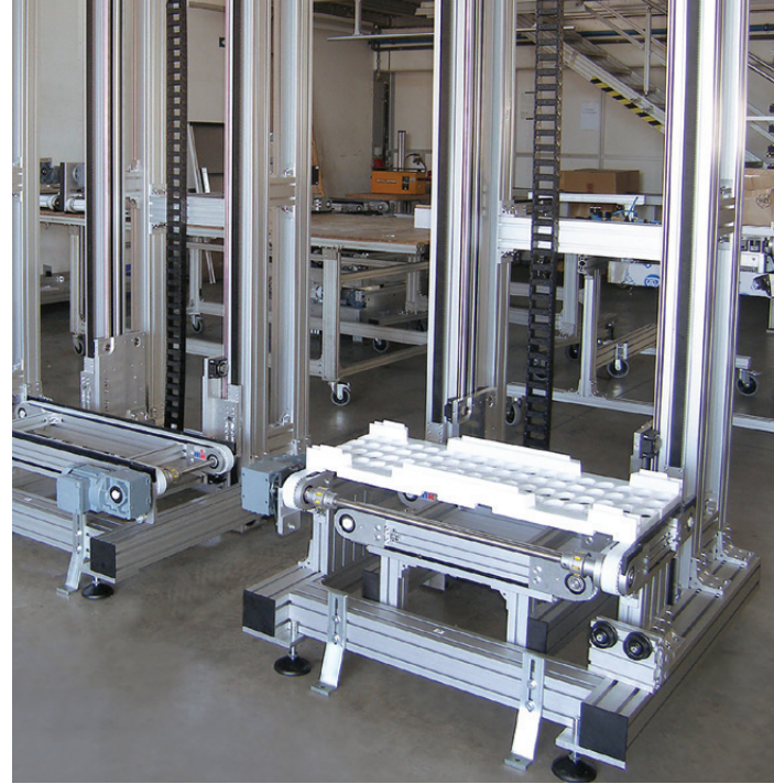
As seen in this example, LZRs are typically used with conveyors to create vertical transfer units, also known as elevators.
