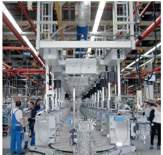
Overhead structure built from Series 40 profiles to support supply lines for assembly workstations
