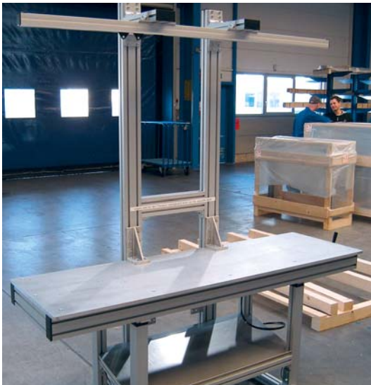
Assembly workstation with crank-operated manual height adjustment, 600 kg load capacity
