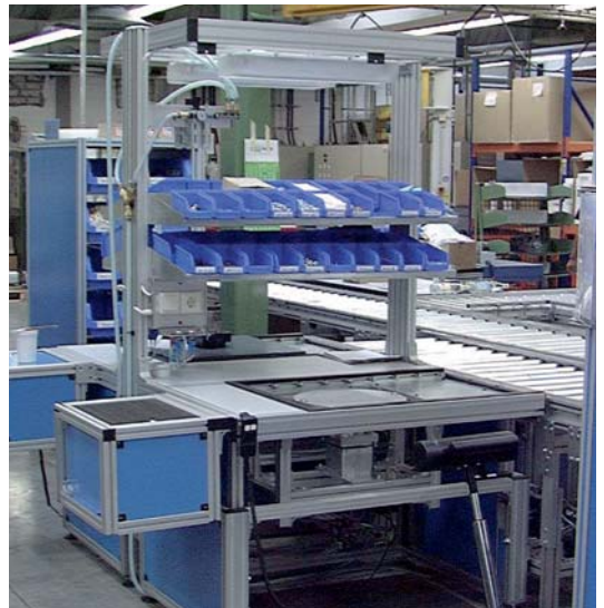
DFT flow line for manufacturing vacuum pumps
