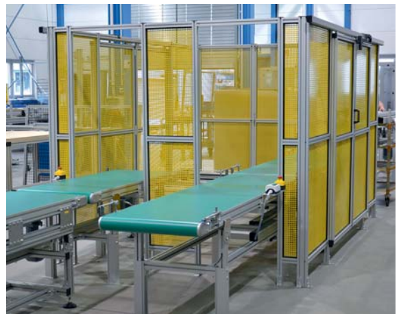
Custom protective device guard made from partitions with powder-coated perforated sheets and sliding doors with solenoid latches
