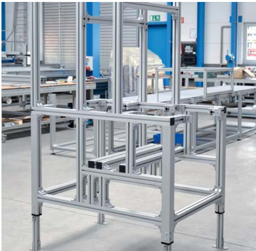
Machine frame made from Series 50 profiles
