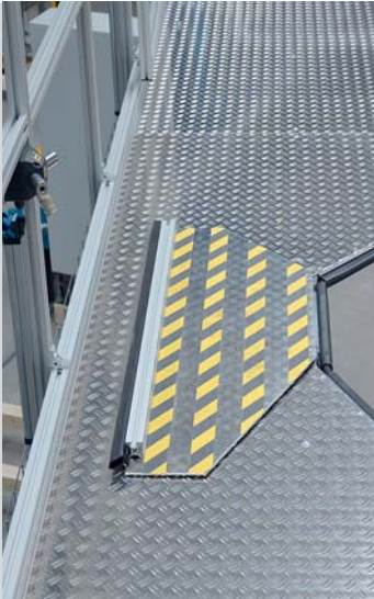
Assembly flap in platform floor with anti-slip covering
