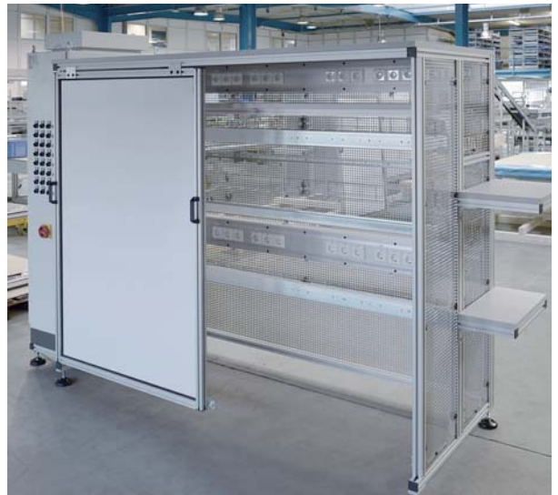
Test bench for pumps with perforated sheet panelling, sliding door and keyboard shelves
