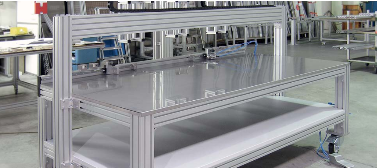
Custom assembly table with linear guide and pneumatic tensioning device
