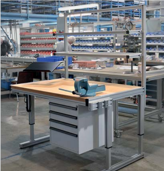
Workstation with electro-hydraulic height adjustment and base cabinet
