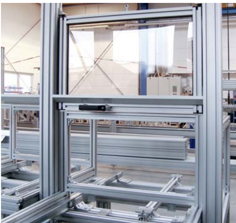
Manual lifting doors with counterweights in the profile, connected by cable and idler pulleys, capable of balancing
