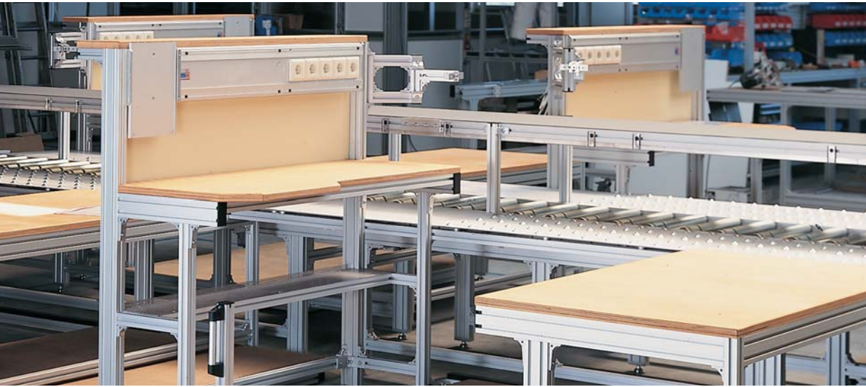
Interlinked industrial workstation with integrated electrical supply and driven roller conveyor
