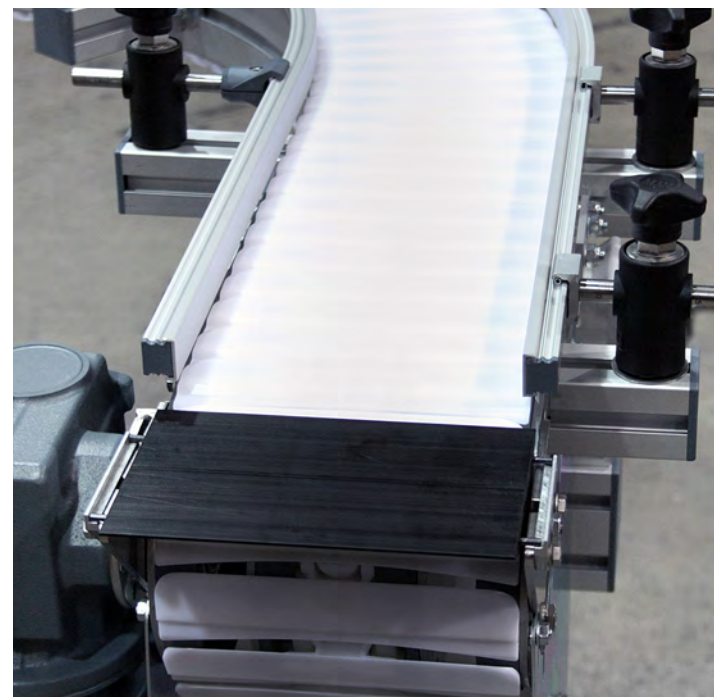
In some applications transfer plates are a more suitable option than the standard roller transfers.
