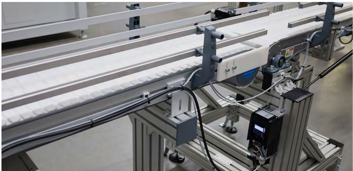
A VersaFlex A29 conveyor system that includes a free-standing lift gate (right side of image) to allow for line access.
