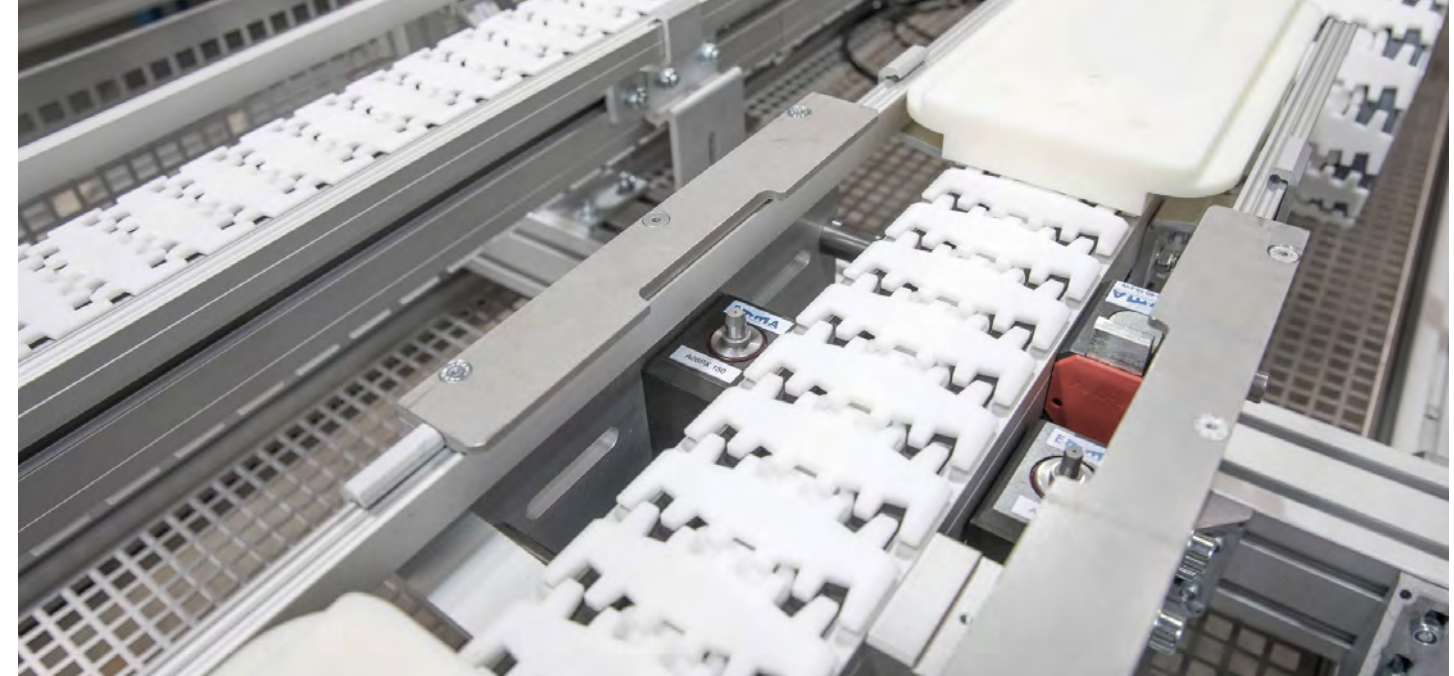
Stop, locate and lift features are fully modular, allowing them to be positioned anywhere along the conveyor line without adjusting the side rails.
