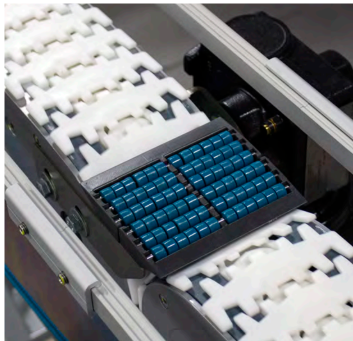
Product transfers, such as the rollers seen here, make it possible to convey products with small footprints between conveyors.
