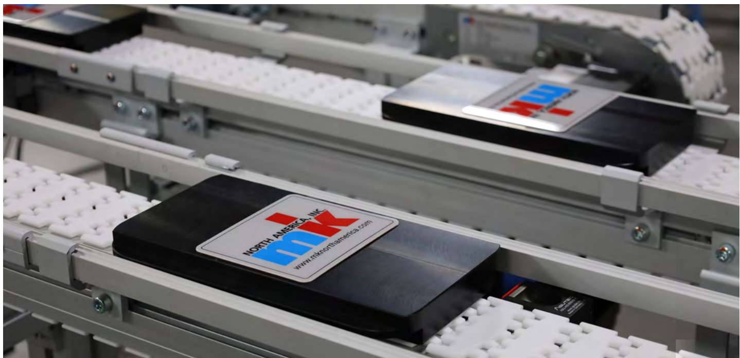
In this example a pallet is about to come in contact with a Pallet Stop. Pallet Stops are used to stop a pallet at a designated location.
