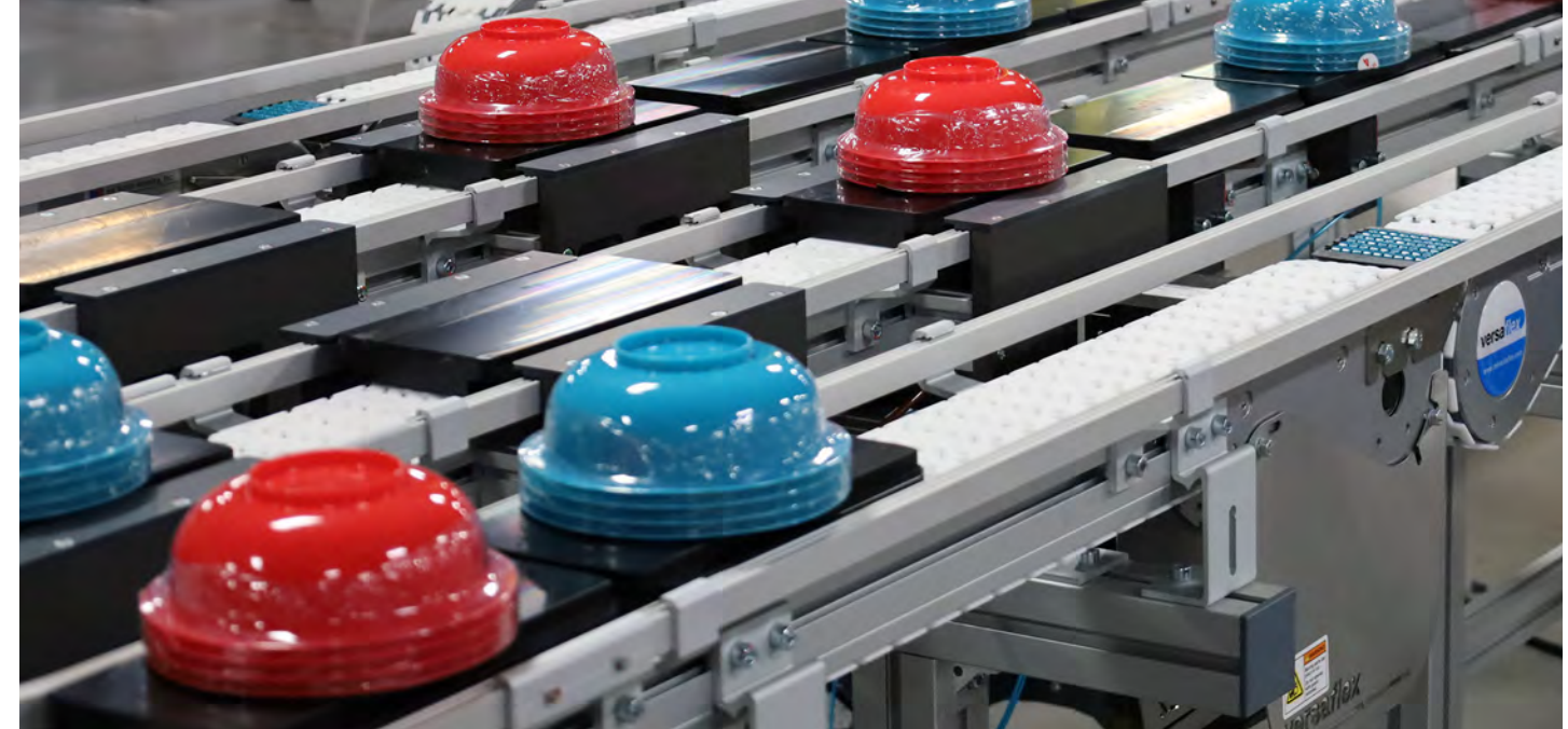
Pallets pass through a number of locating stations along a recirculating conveyor line.
