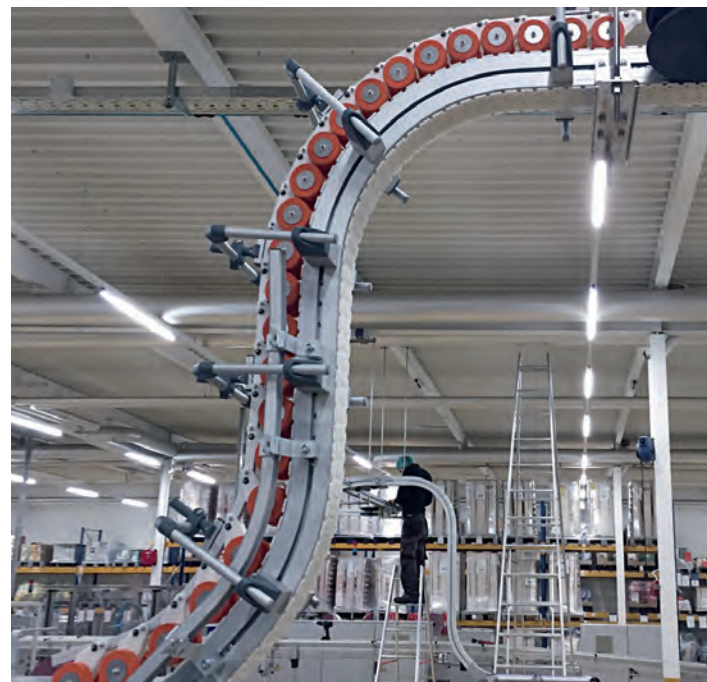
Vertical product conveying is possible for the VersaFlex. In this application guider-rollers above the chain help contain the product.
