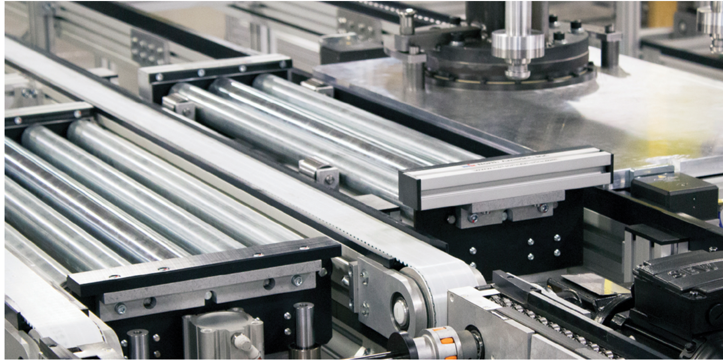
A ZRF-P 2040 Timing Belt Conveyor with an SRF-P 2012 Accumulating Roller Chain Conveyor receive pallets from an RBM 2012 Lift and Transfer.
