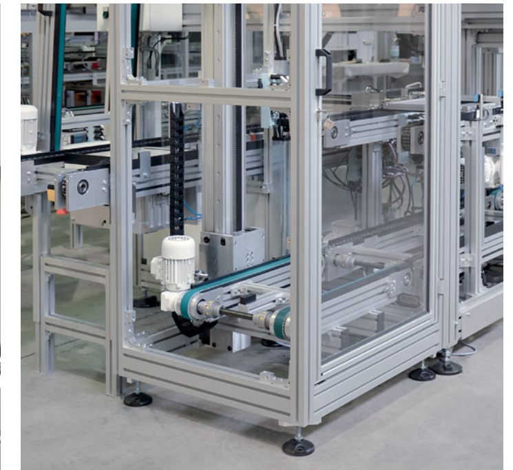
mk offers a wide variety of standard and custom Vertical Transfer Units, as well as electrically driven options.
