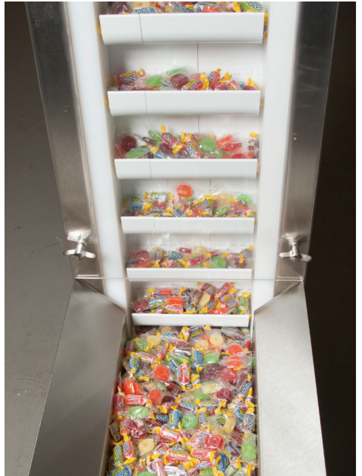
Vertical conveyors can take product from ground level, often out of a hopper, and carry it vertically to the next stage or process.
