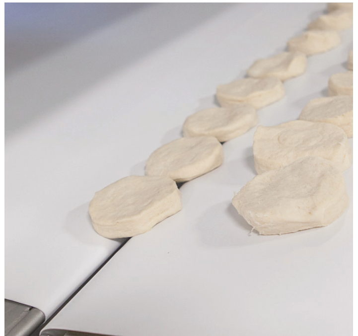
Tight nose bars allow for the most delicate products to easily transfer between conveyors.
