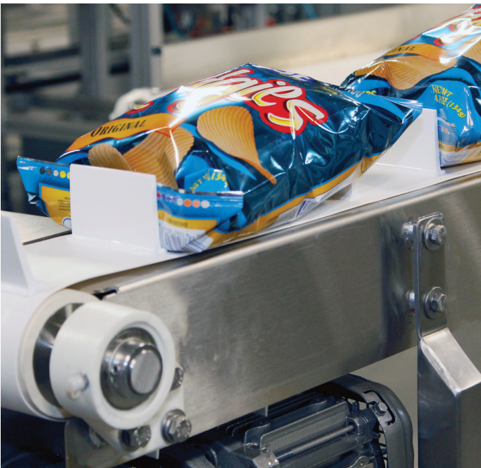
Cleats on belts can be used for a wide variety of applications, including creating desired space between products.
