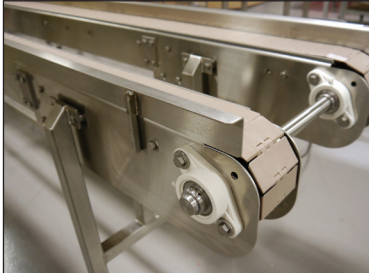
A CTF-200 Flat Top Chain conveyor, constructed in a multi-lane set-up.
