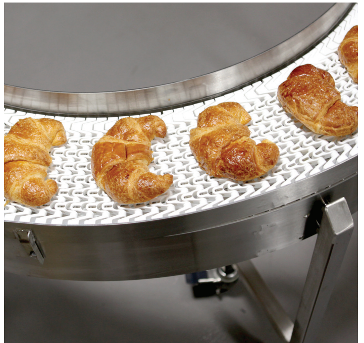
Croissants travel on a curve conveyor to a wrapping station. This conveyor features removable side rails and casters.
