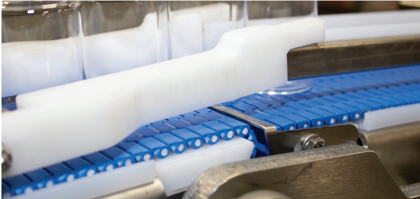
Delicate parts are transferred from one conveyor to the next using tight nose bars and a small transfer plate.
